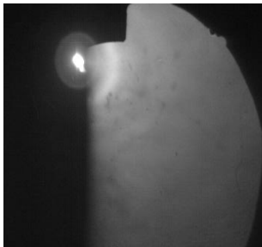
Figure 2. The RHEED diffraction picture from an 82 Å thick Bi film on HOPG. At least one diffuse ring is clearly visible.
